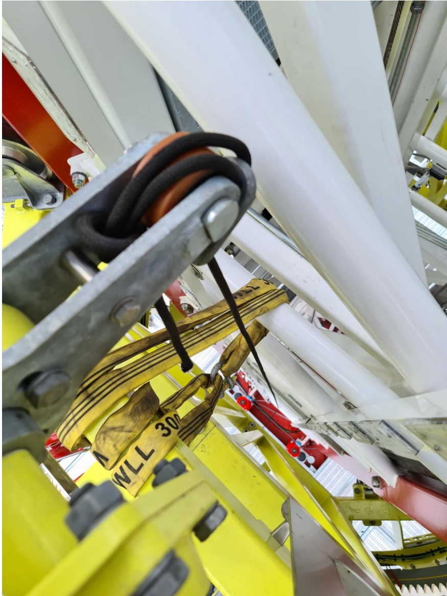
Figure 5-33 Rope on the release mechanism
