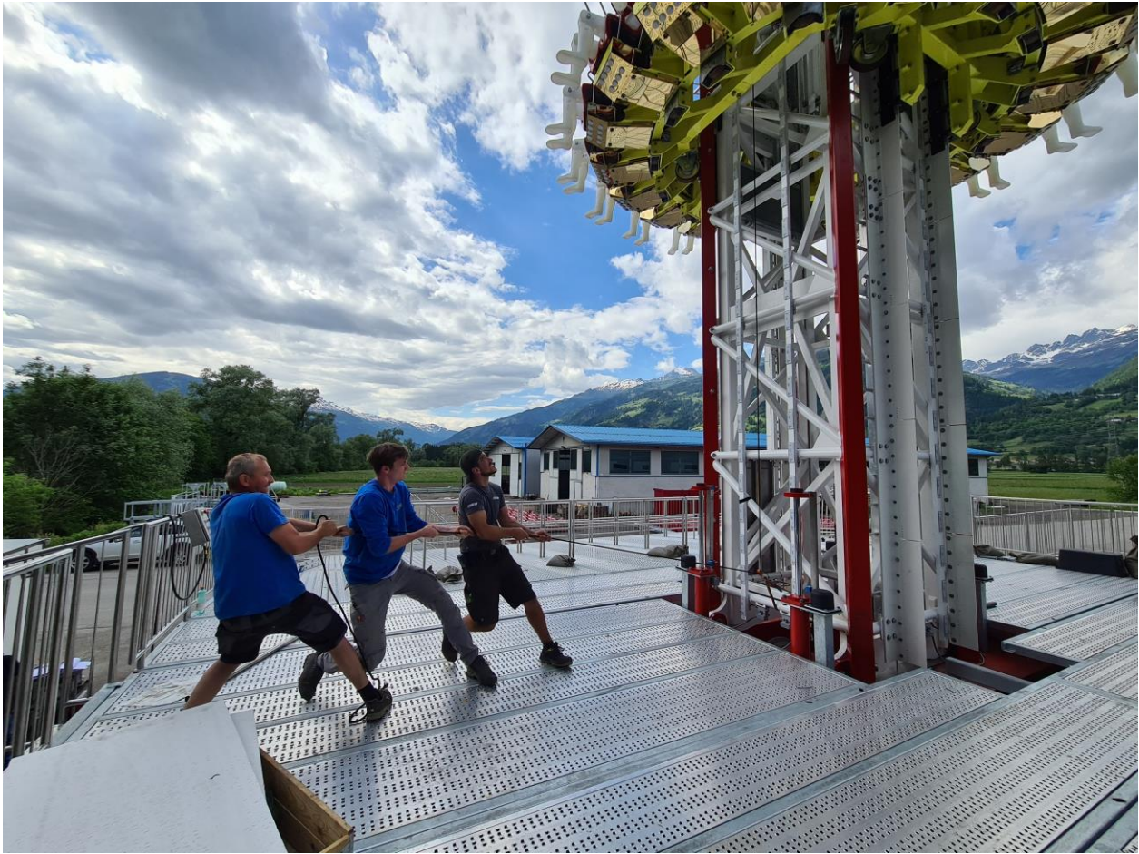
Figure 5-35 Release gondola by pulling the rope
