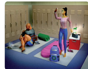
General population: 20 sq. ft. of space is available for one person and all necessary items.
